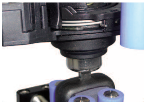
Measuring torsion-sprung lock effort
