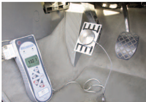
Pedal force testing
