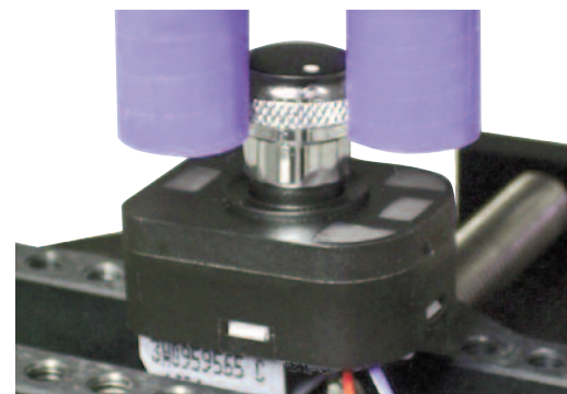
Torque testing of rotary switch
