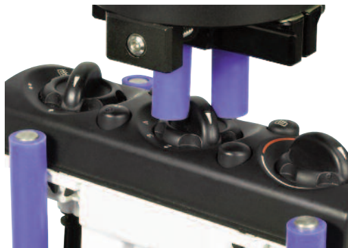
Rotary controls under torque test
