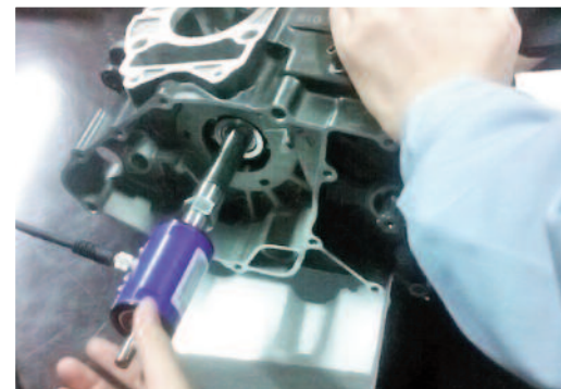
Torque testing a motor shaft
