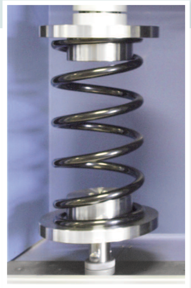
Suspension spring under compressive test on a Mecmesin MultiTest 25-i system
