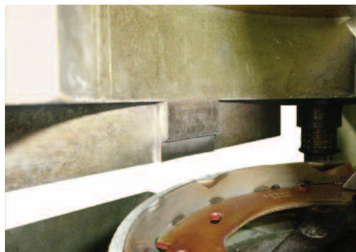
Measuring shear strength of brake linings
