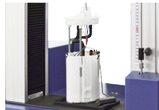
Spring testing in a fuel pump assembly
