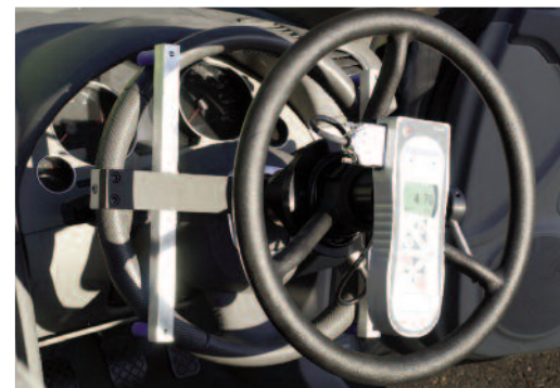
Testing torque with or without power steering
